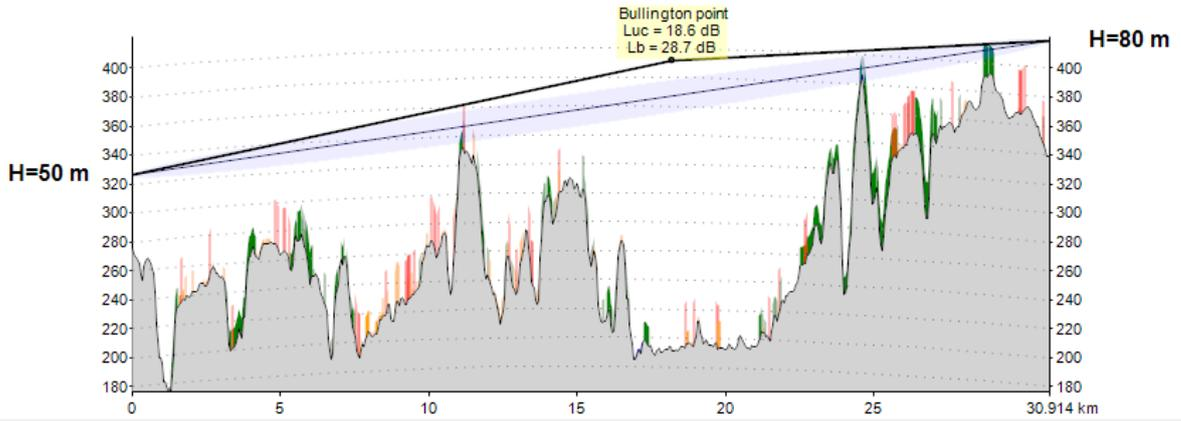
Diffraction analysis according Rec. ITU-R P.526-15
