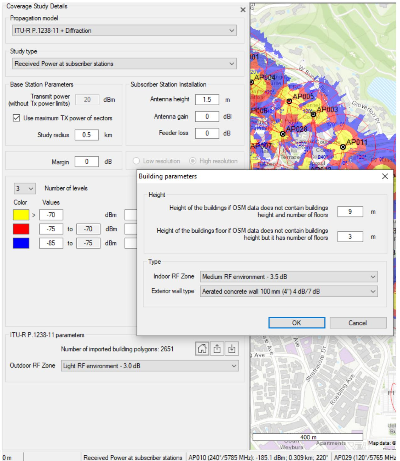
*ITU-R P.1238-11 + Diffraction model parameters*
