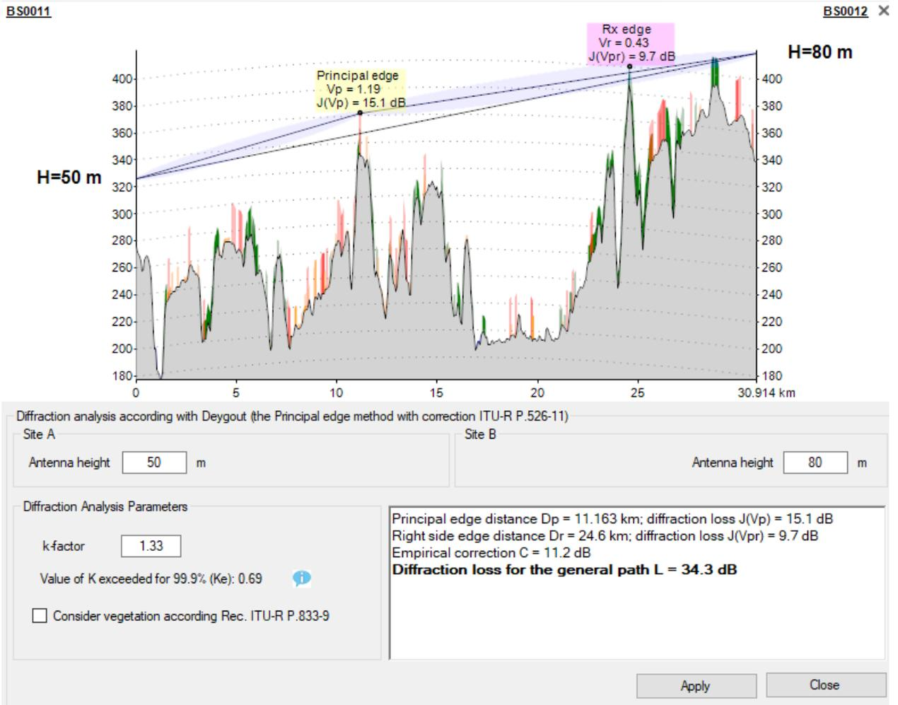
*Deygout Diffraction Loss Analysis Rec. ITU-R P.526-11*
