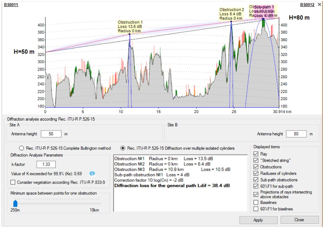
Analysis of diffraction losses by the method of isolated cylinders according to Rec. ITU-R P.526-15
