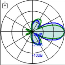
Antenna cross polarity isolation, dB
